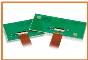
FH58/M Space-Saving, Top/Bottom Contact Pitch: 0.2mm (FH58M: 0.25) Height: 0.9mm Depth: 3.1mm (FH58A: 3.4) Pin Count: 7-71pos. (Under Development: 81) Rated Current: 0.2A
